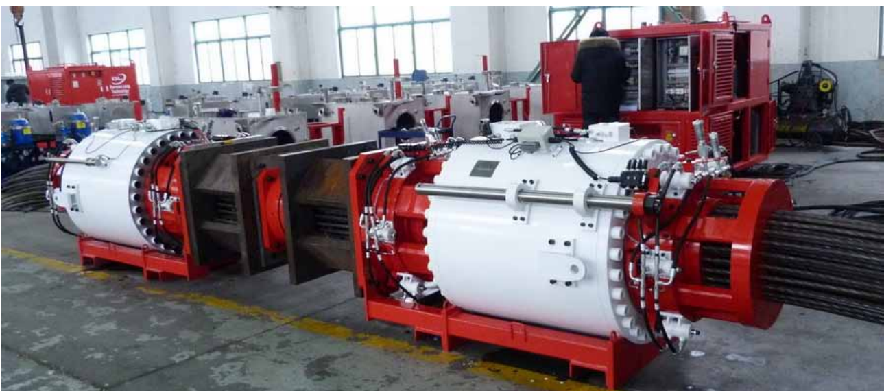
2 No DL-S836 strand jacks during 125% load testing in the factory, with transport frames
