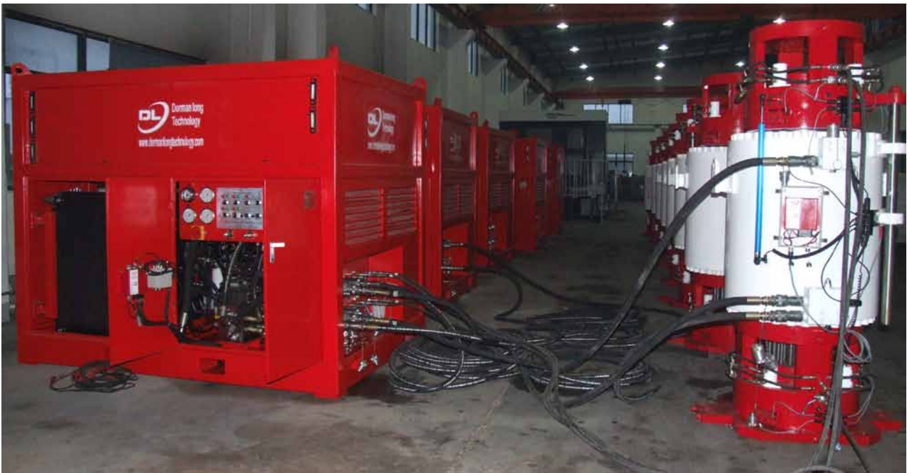
DL-L120/2/300/D Diesel powered hydraulic power packs and DL-S588 strand jacks
